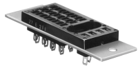
Flange Mount Socket Solder terminal socket with tin-plated terminals and grounding strip pre-assembled on .065" (1.65mm) steel mounting plate. Requires only one chassis cutout.
